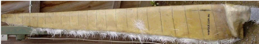
Figure 6. Blade after being covered in chop strand matt fibreglass
