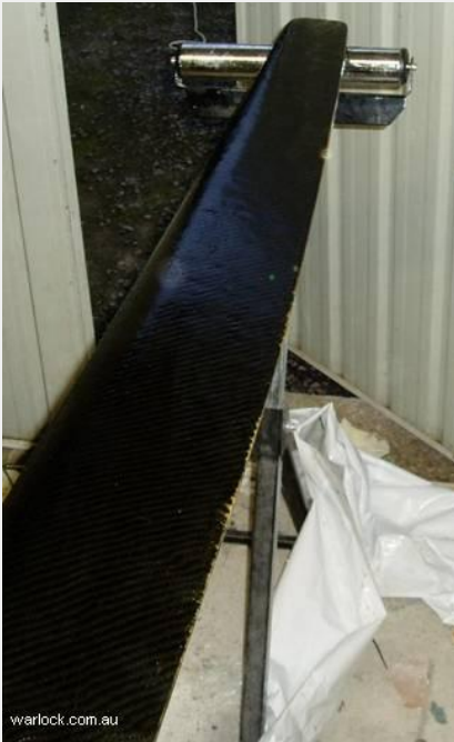
Figure 9. Blade after sanding the carbon fibre
