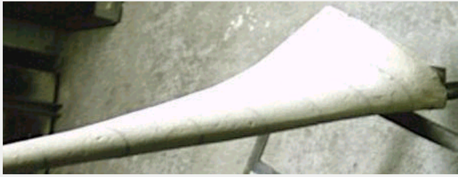
Figure 5. Polyurethane foam blade after sanding
