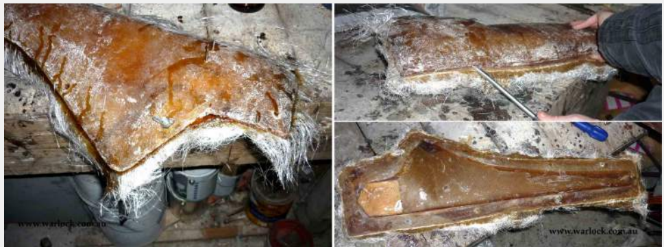
Figure 8. A moulded blade ready to be cured (left). Breaking the cured mould apart (right).
