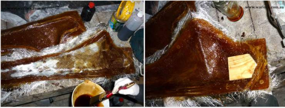
Figure 7. Half moulds being filled with glass and soaked in resin (left). A wooden hub is fitted at the end (right).
