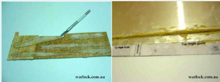
Figure 1. The airfoil shapes were constructed using balsa (left). The root and angle-guide were made from tin sheet and wire (right).
