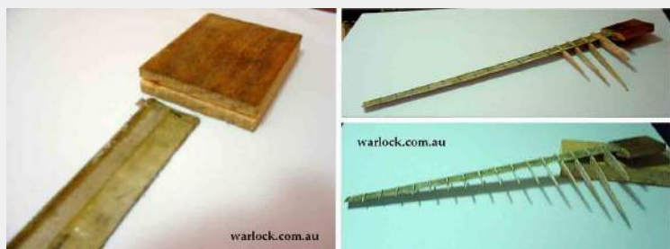
Figure 2. The root section glued to the hub (top). The balsa airfoil shapes glued along the root (bottom).
