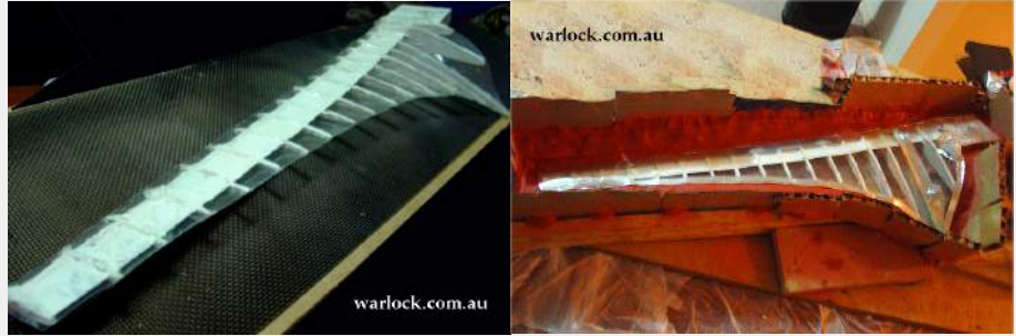
Figure 3. The gel coated skeleton with plastic sheet glued to the balsa shapes (left). The final blade skeleton with border made of modelling clay (right).
