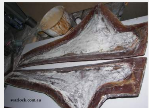
Figure 6. Making the fibreglass mould (left) and waxing before use (right).
