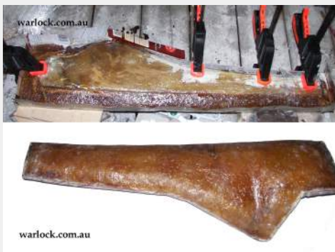
Figure 6. Making the fibreglass mould (left) and waxing before use (right).
