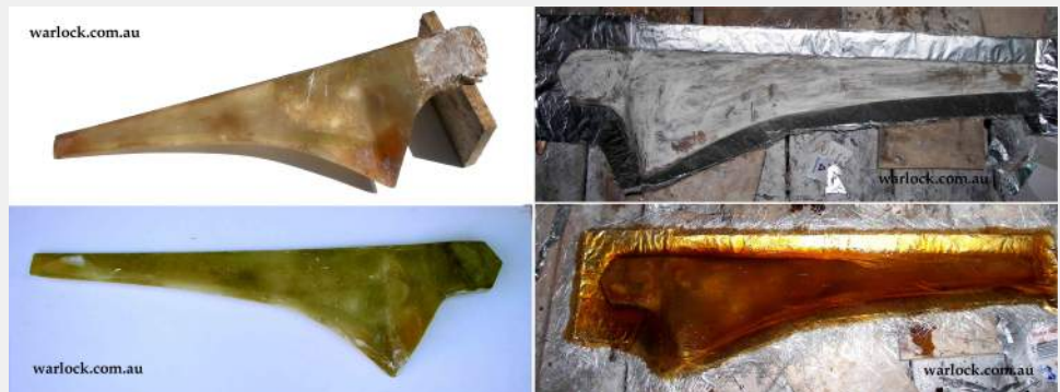
Figure 5. The fibreglass blade from the plaster mould (left). Making the fibreglass mould from the blade (right).
