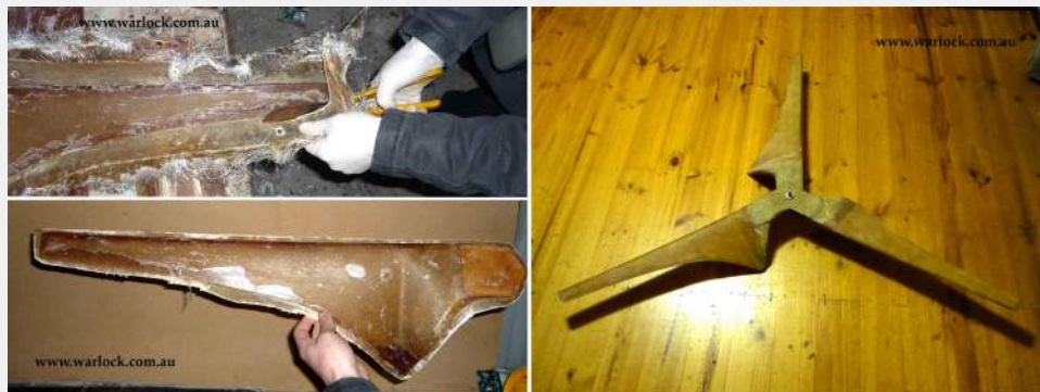
Figure 9. Fibreglass blades from the mould (left). The finished 3 blade set (right).
