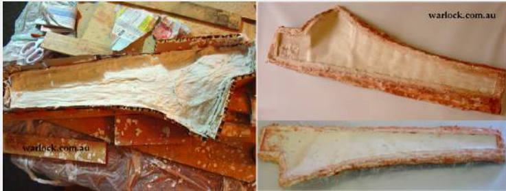
Figure 3. The gel coated skeleton with plastic sheet glued to the balsa shapes (left). The final blade skeleton with border made of modelling clay (right).
