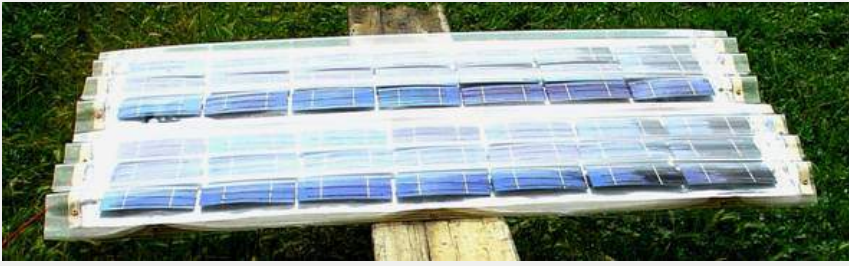
Figure 9. The corrugated dome catches additional tangential light which would normally be lost with a flat panel
