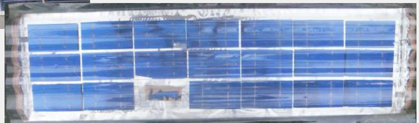
Figure 14. Solar panel with damaged cells bypassed
