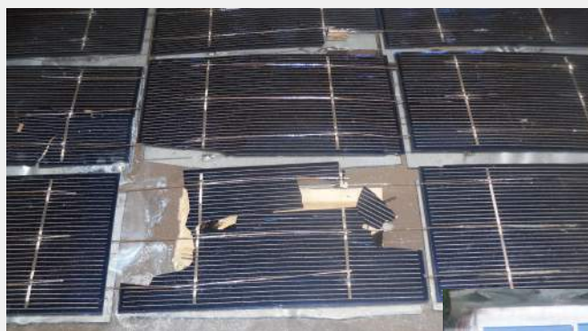
Figure 14. Solar panel with damaged cells bypassed
