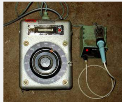
Figure 2. A temperature controlled soldering iron using a variac
