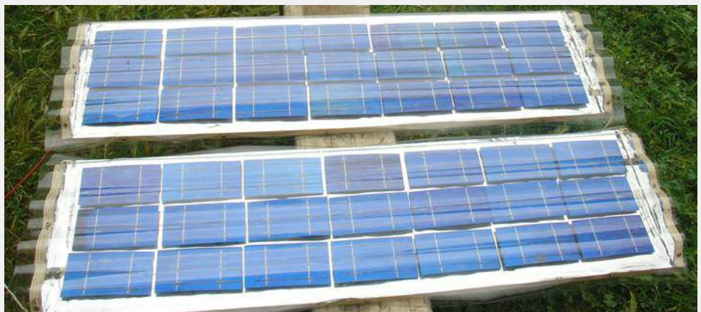
Figure 8. The polycarbonate sheet screwed to the wood
