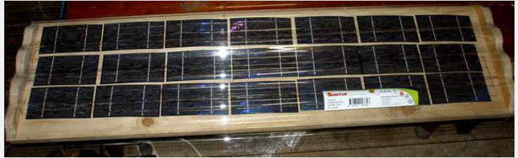
Figure 5. An enclosure constructed using wooden ends to fit the corrugated polycarbonate sheeting over the top of the base
