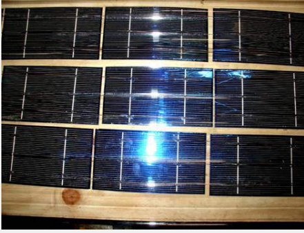
Figure 4. The cells soldered in series in three rows of seven on top of a wooden base
