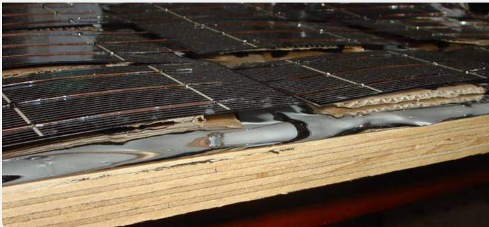
Figure 7. The cells glued to shock absorbing cardboard
